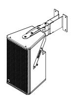
The HPI 8i can be flown in a permanent installation by attaching the designed flying hardware. The HPI-8i can be wall mounted or hung in a flown installation using the flying fitting accessory. For more information, see the Quest HPI flying hardware manual.
