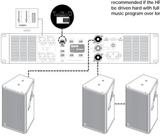
make more amplifier power available for clean vocal reproduction for full range sound, set the high pass filter to 80Hz
